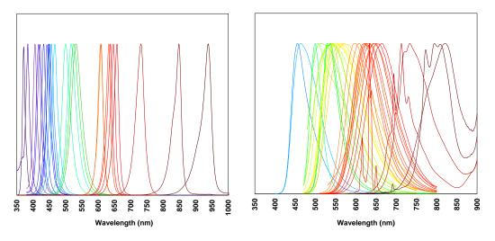
Figure 3. Available spectra for semiconductor and phosphor-converted LED.
