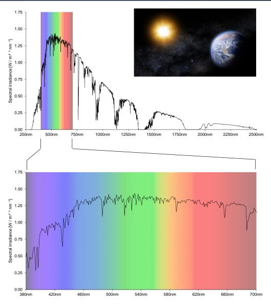
Figure 1. AM 1.5 standard spectrum (direct + circumsolar) in the range of 250nm-2500nm and 380nm-700nm.
