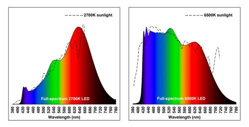
Figure 4. 2700K and 6500K natural light spectrum LED for white light bases.
